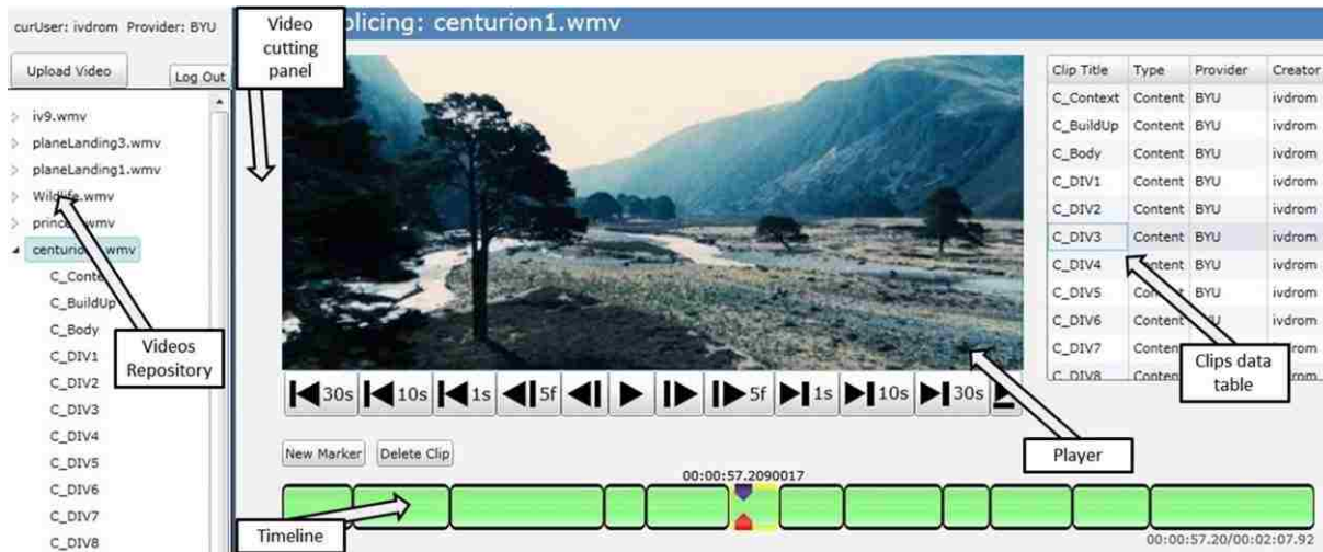
Figure 21 Video Editor tool. Left: clips repository, right: slicing tool and clips data table, bottom: timeline
